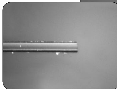
Check profile of fiber for dirt and debris
