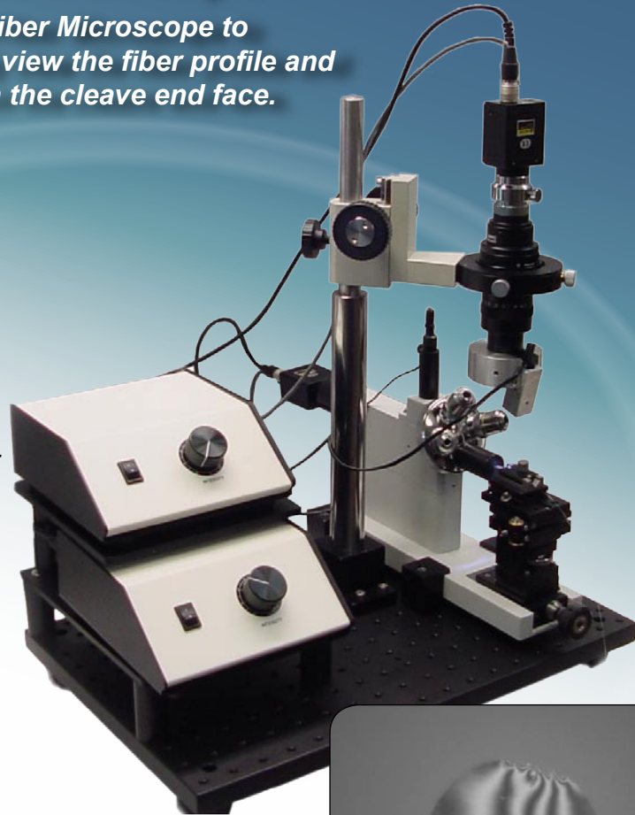
View fringes to check cleave angle
