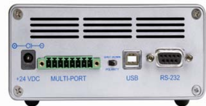
Rear View shows (from L to R): universal power input, multi-port input, USB 2.0 input, RS-232 input
